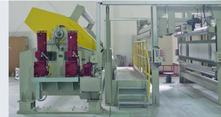
The turret unwinder is designed for 5.600 mm wide and heavy technical textiles. The fabric is fed into the turret winder by means of a crane. The steel winding cores are taken up via automatic bearings.
